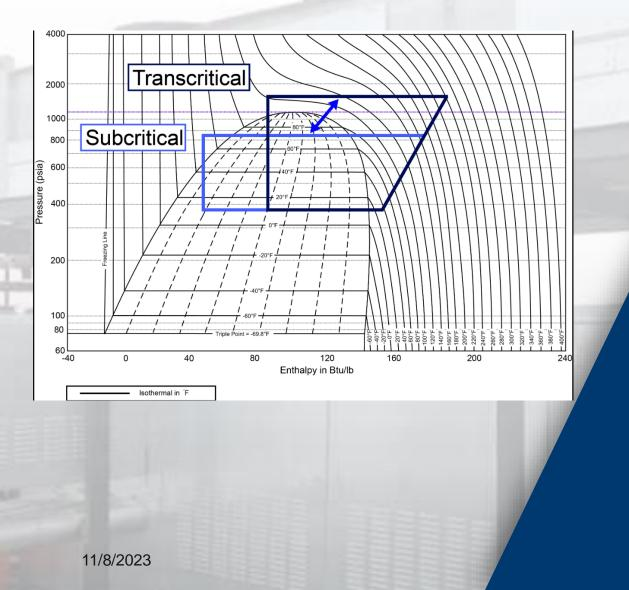
In Sub-Critical operation, the condenser does just that, condenses the refrigerant by simply removing heat.
